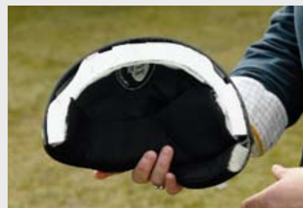
This hat has been impact tested, you can see the dent in the polystyrene. If it was struck again on the same spot, it would not absorb the impact
